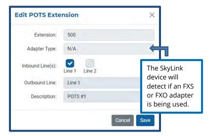
Under the Inbound Line(s) field, tick each box to allow calls to both Line 1 and Line 2. Deselect both lines to block calls from ringing to an extension. **NOTE**: If you are not receiving calls to your extension, ensure one or both lines are selected here.
