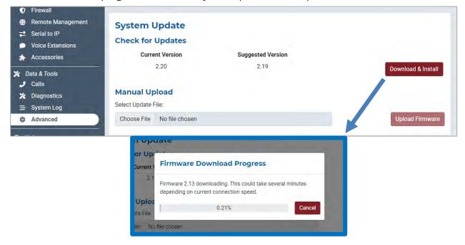
Alternatively, click the 'Choose File' button under the Manual Upload section. Locate and select the appropriate .tpz file, then press 'Upload Firmware' to start the firmware upgrade process.
