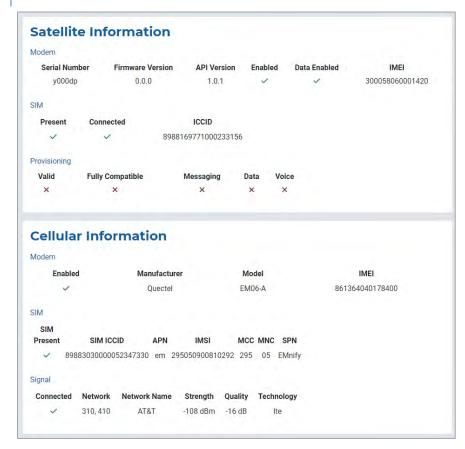
Use the check marks in these sections to verify that your satellite and cellular capabilities are enabled. Data related to the satellite and cellular modems, SIM cards, satellite provisioning, and cellular signal are available here as well.
