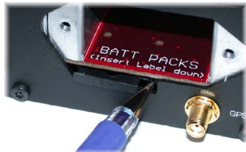
Eject card tray (and remove) using a pen
