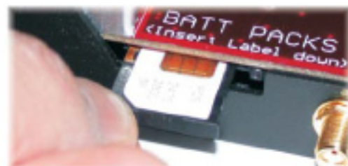
C. Carefully insert SIM in tray with contacts (chip side) facing UP.
