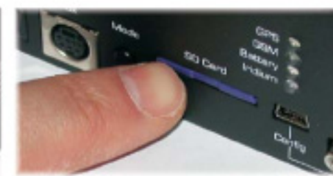
A. Insert SD-Card: contacts facing up B. SD-Card will "click" into position
